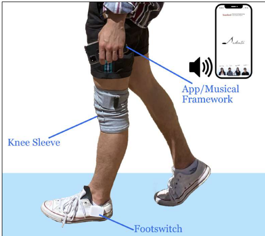
Figure 11: Full System Design made of the footswitch, knee sleeve, and app/musical framework.
