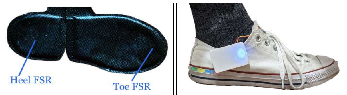
Figure 13: Footswitch insole with FSRs (left) and footswitch insole and battery case attached to the shoe (right).
